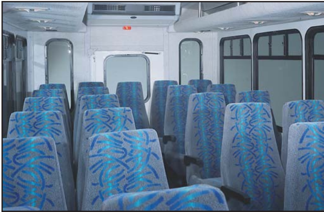
A sample Allstar interior, shown here with 25 passenger seating, overhead luggage rack and rear air conditioning.
